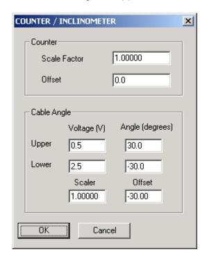
If you determine that the incoming cable count is incorrect, possibly due to a miscalibration of the counter itself, a compensating Scale Factor can be entered in the Counter section. An offset value can also be entered. This offset value will be added to the scaled cable count.
