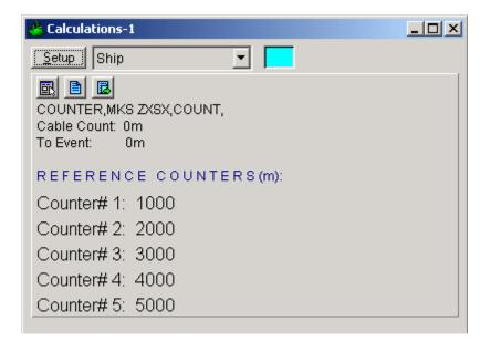
Once the Calculations window has been opened and configured, the five reference counters can be modified using the Reference Counters page of the Configure Counter dialog. (Note: the Configure Counter dialog can be directly accessed from the Calculations window by clicking the icon in the Calculations window.)
