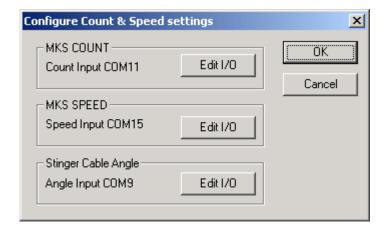
Click the Config button for each one of the data types to open the standard Device I/O Parameters windows. Enter The I/O parameters for each data type and exit with OK.
